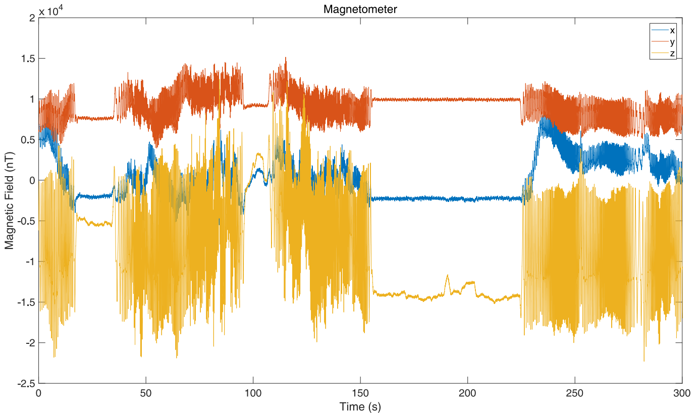
Fig. 3. Magnetometer measurements from electric bus
