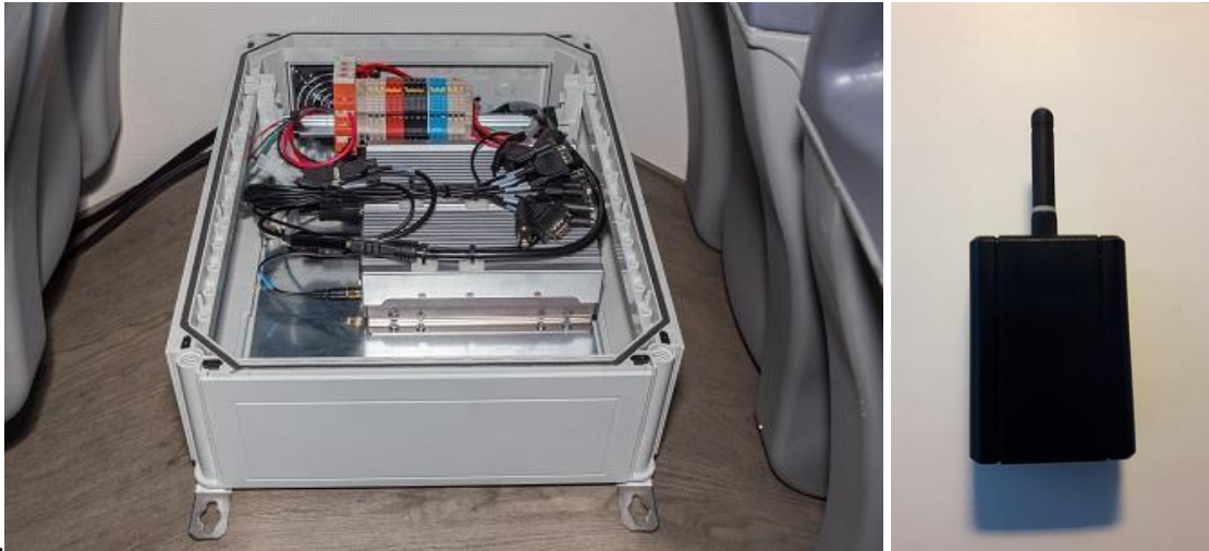
Figure 5 - The OMEC gateway unit box ready for installation (left) and LoRaWAN connected TinyNode measurement hub (right).
