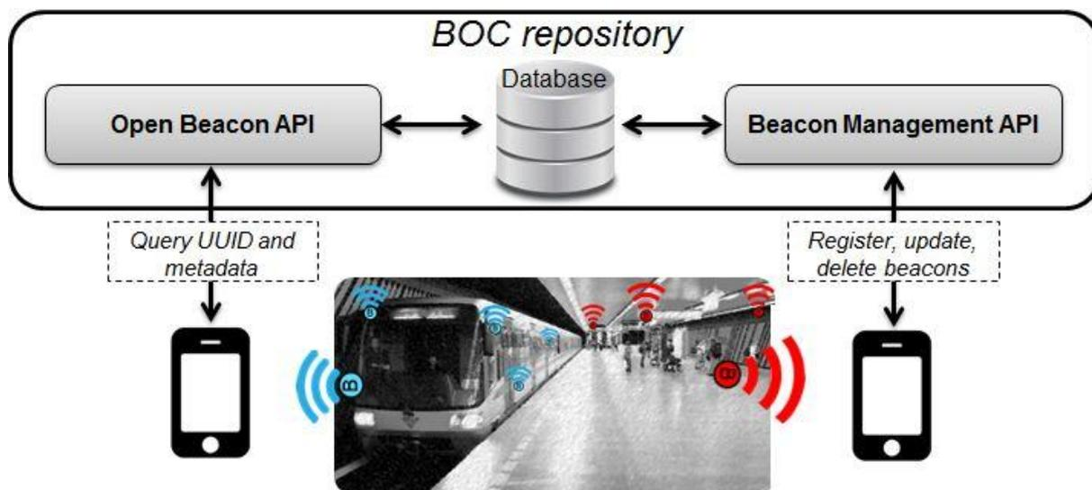
**Figure 3. High-level architecture of the BOC system.**
